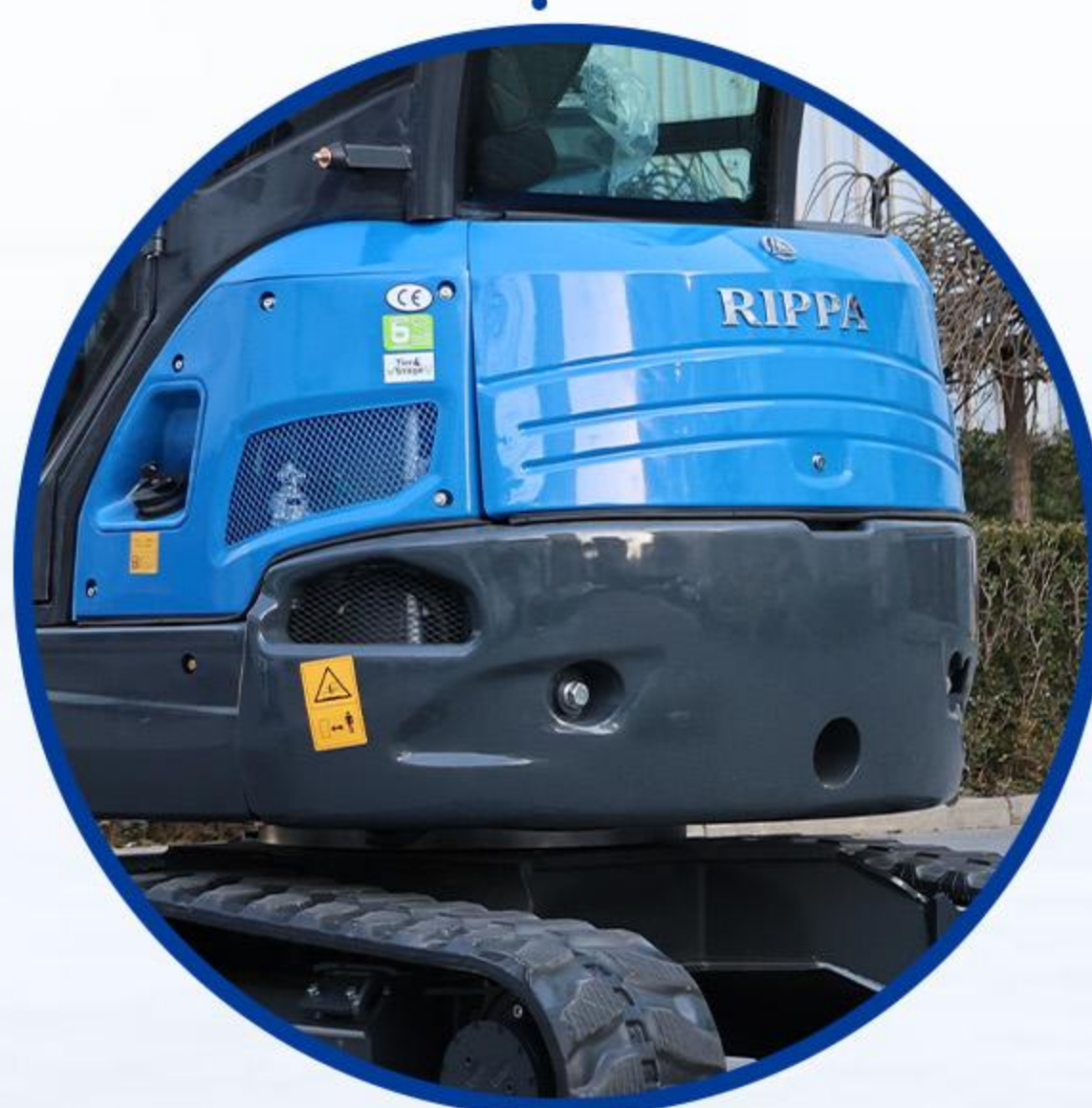
Counterweight-Real weight : 3.2Ton
