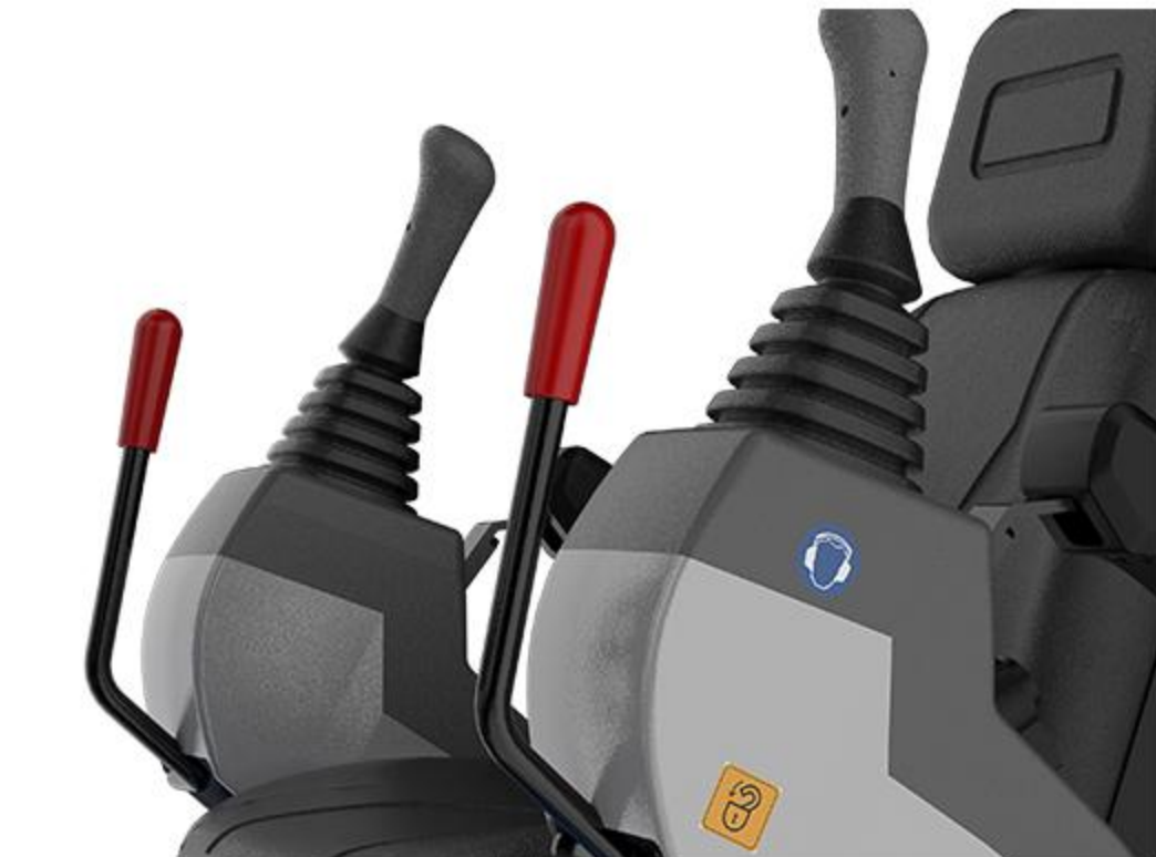
2 Operation Lock Lever It is equipped with an engine neutral start function that prevents the engine from starting unless the operation lock lever is in the raised position.
