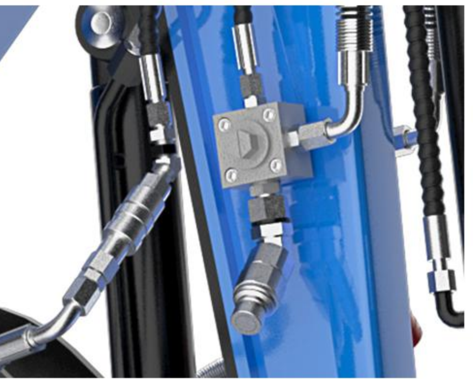
9 Four-way oil pipe Can be equipped with various accessories
