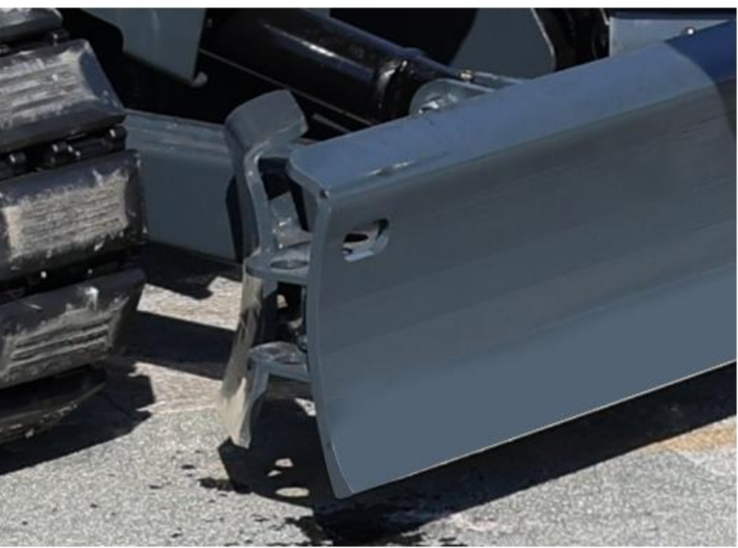
7 Extended bulldozer blade The width of the dozer blade can be easily extended by removing and attaching the pin.
