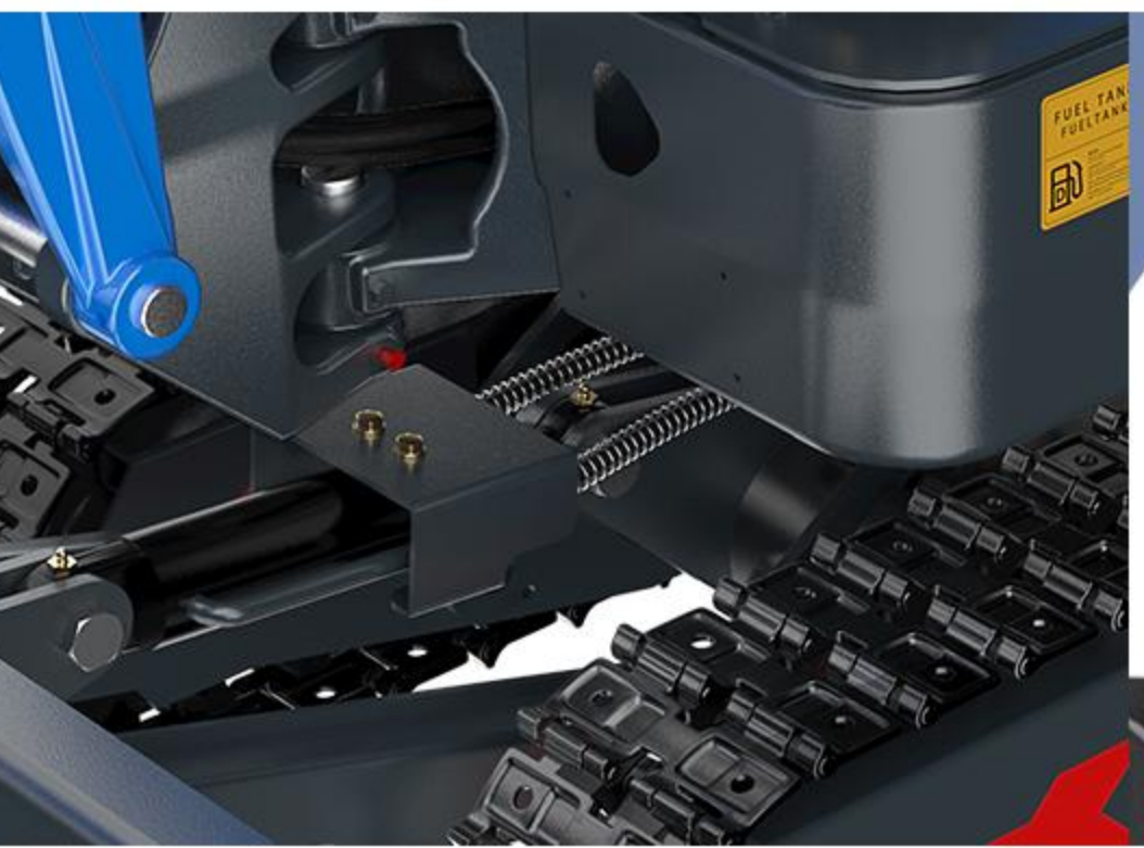
8 Split Dozer Hose In the event of unexpected damage, the hose can be easily replaced.
